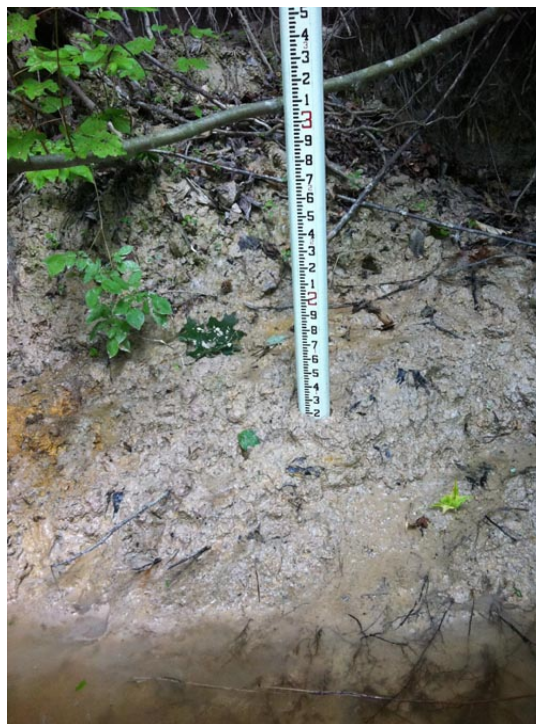
Photos 3.1 and 3.2 – Eroding bank downstream side of Magnolia Road and plastic clay layer at toe of bank
