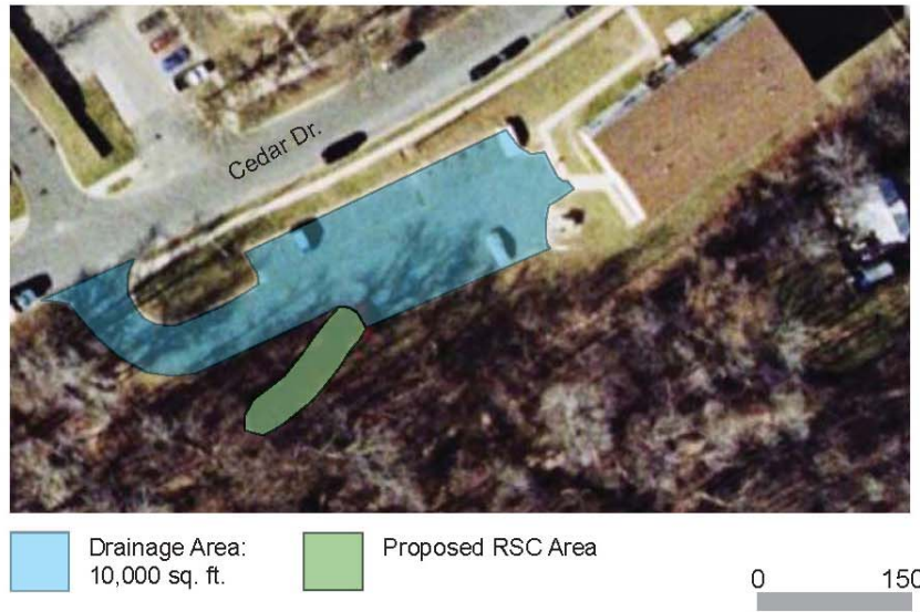
Figure 3-14. SBL – Regenerative Stormwater Conveyance
